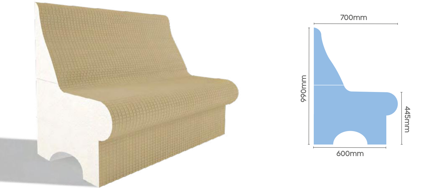
Example showing standard modular seating profiles used to create bespoke seating designs. Profiles can be cut to suit site specific dimensions.
