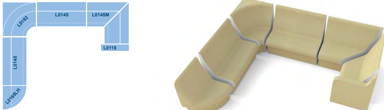
Example showing standard modular seating profiles used to create bespoke seating designs. Profiles can be cut to suit site specific dimensions.
