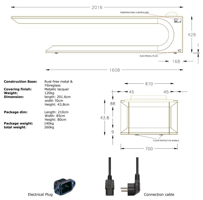
If fixed installation is needed Cleopatra could be delivered without wheels. In this case the connection could be be hidden in the base.
