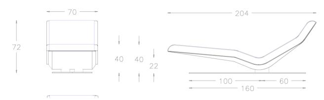
Construction Base: Rust-free metal Construction Base covering: Fibreglass Covering finish: Metallic lacquer
